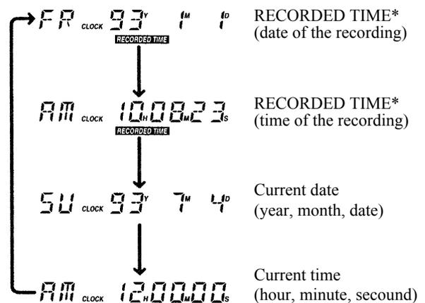
\*The RECORDED TIME will not be displayed while the unit is in the recording, recording monitor, or pause mode.
