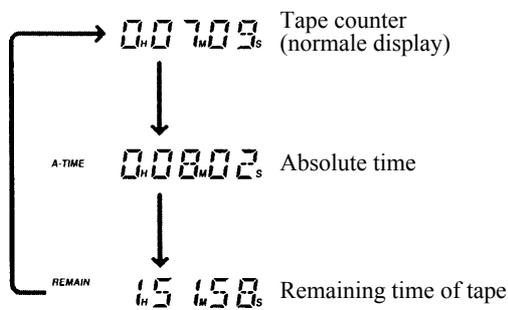
**To reset the tape counter (normal display) to 00H00M00s**
