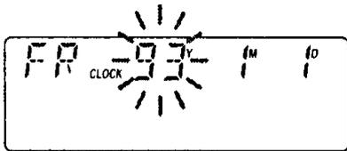
2 Press the COUNTER/- and RESET/+ buttons to set the year digits, then press the CLOCK/SET button.
