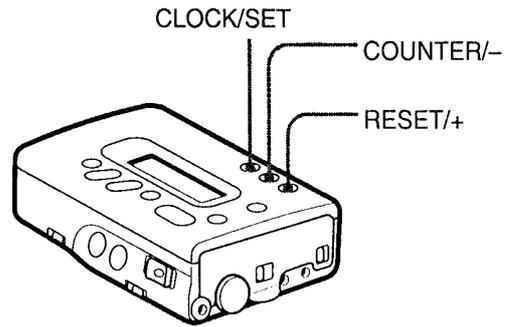
5 Press the COUNTER/- and RESET/+ buttons to set the day, then press the CLOCK/SET button.
