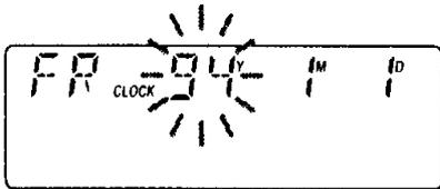
3 Press the COUNTER/- and RESET/+ buttons to set the month digits, then press CLOCK/SET-button.
