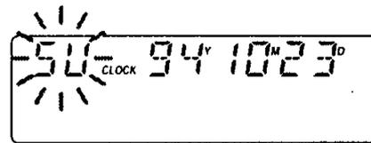
6 Repeat steps 2 to 4 to set the correct current time (hour/minute/second). The second digits change to "00" when the COUNTER/- or RESET/+ button is pressed and the clock starts activating when the CLOCK/SET button is pressed. Therefore, synchronize the clock by pressing either - or + button with the radio time-signal etc.
