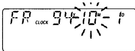
4 Press the COUNTER/- and RESET/+ buttons to set the date digits, then press the CLOCK/SET button.
