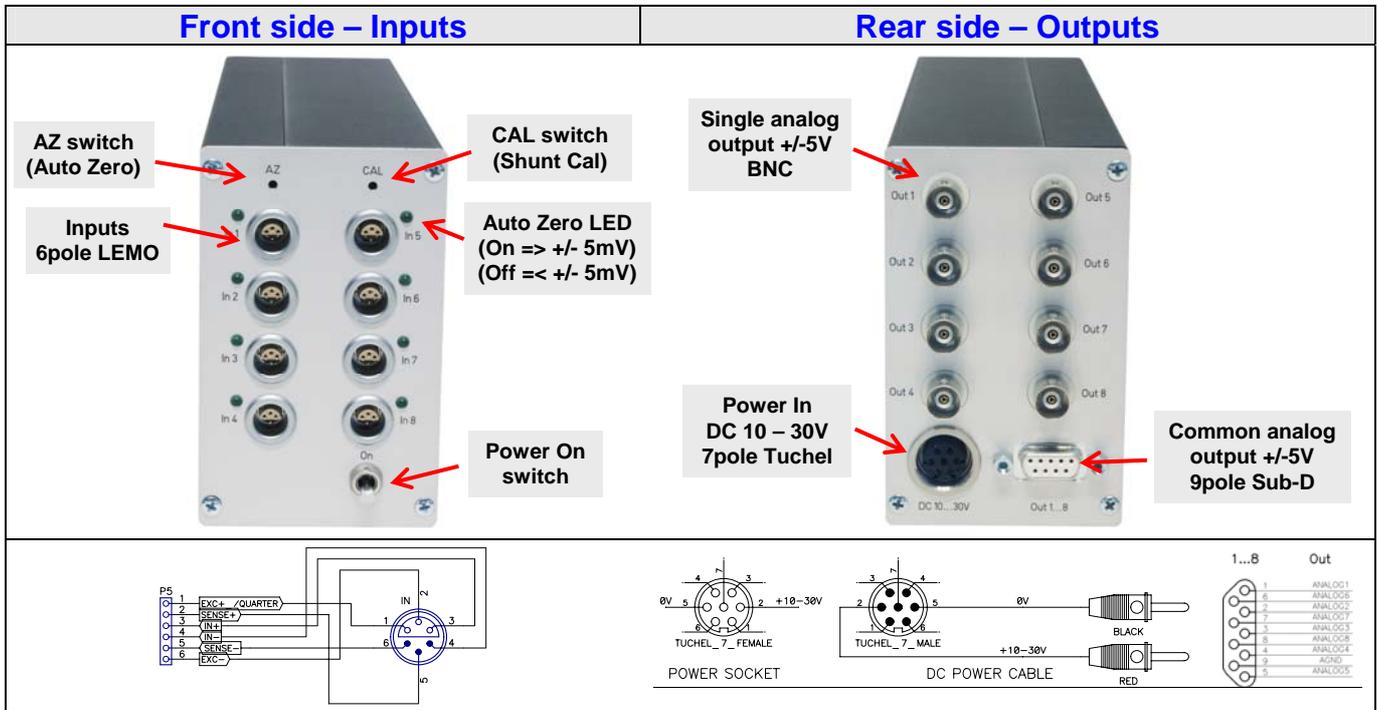
Dimensions: 65 x 105 x 250 mm, Weight 1.5kg, Powering: 10-30V DC, Operating temperature range: - 20°C ... + 80°C
