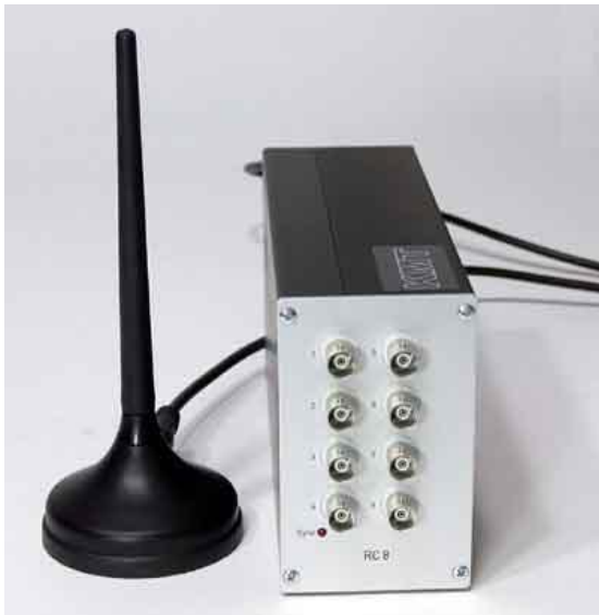
Figure 5.1: MT32, 8-channel telemetry decoder with 8 analog signal outputs (+/-5V)
